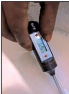
Digital thermometer – most reliable, but also the most expensive temperature control help. Occasionally needs a new battery. Recommended for the serious cheese maker
